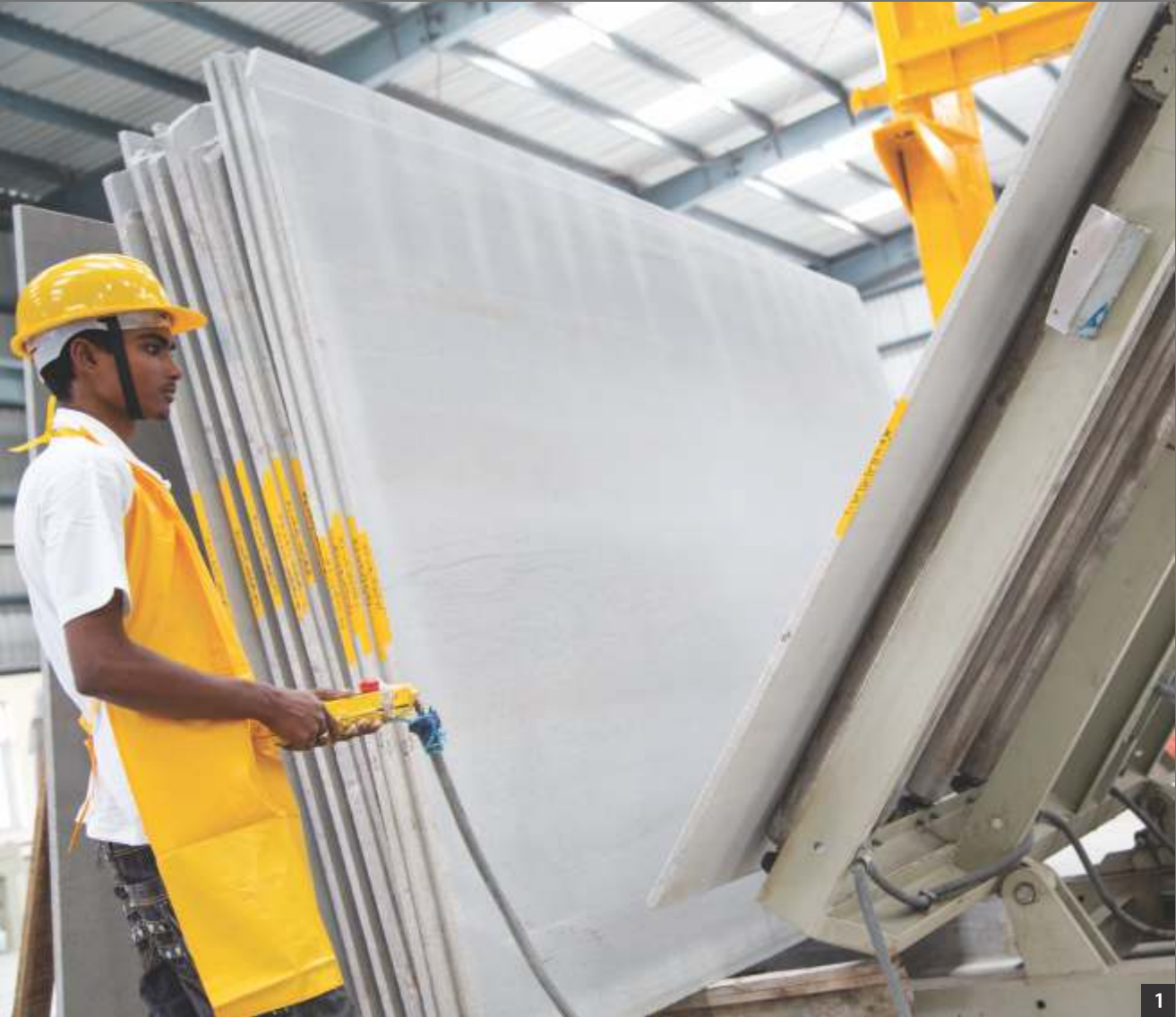
1. Granite Slab Handling Machine 2. Granite Quarry at Yelagiri Hills
