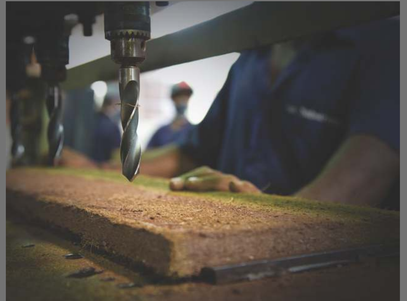
Providing Grooves in Cocopeat slabs
