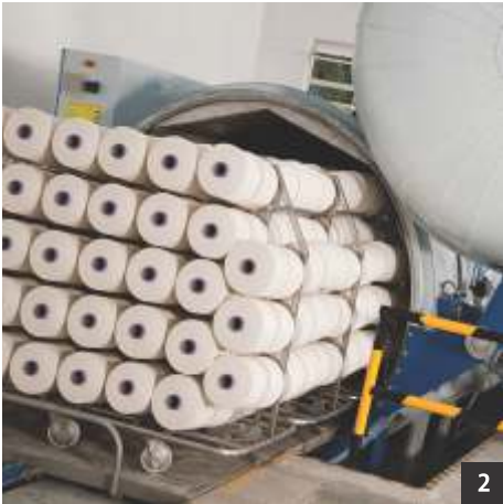
1. Rieter E66 Combers 2. Elgi Yarn Conditioning Plant 3. Uster Tester 5
