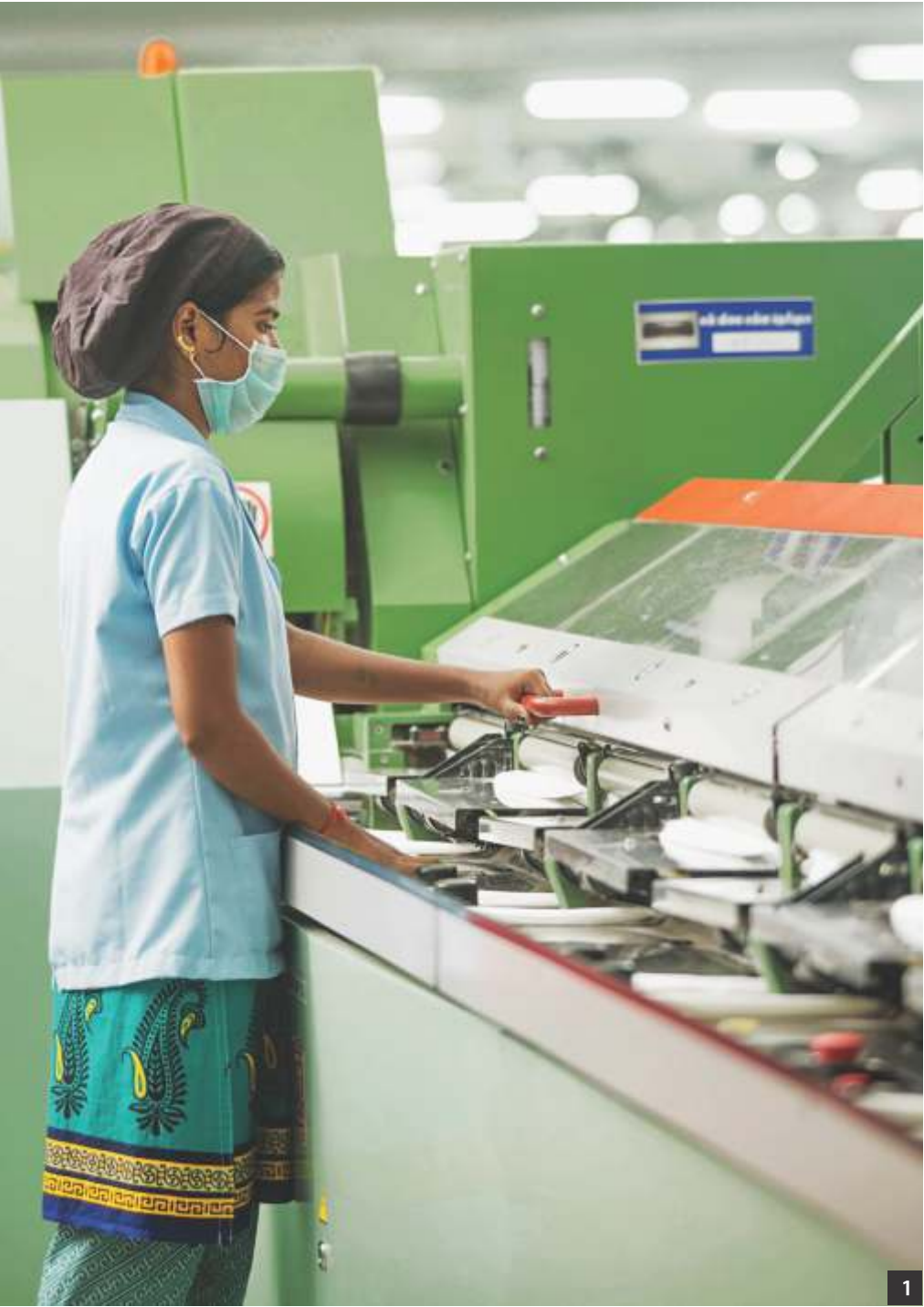
1. Rieter E66 Combers 2. Elgi Yarn Conditioning Plant 3. Uster Tester 5
