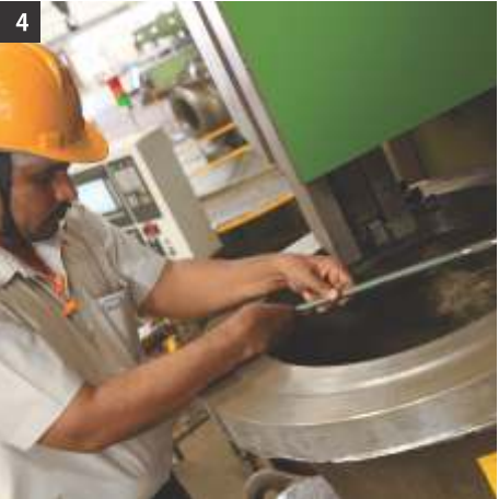
4. Vertical Turning Lathe with CNC attachment
